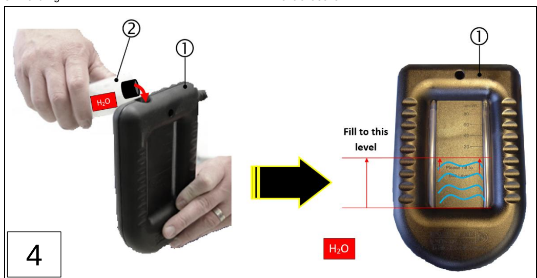
1: U- Rohr- Manometer
