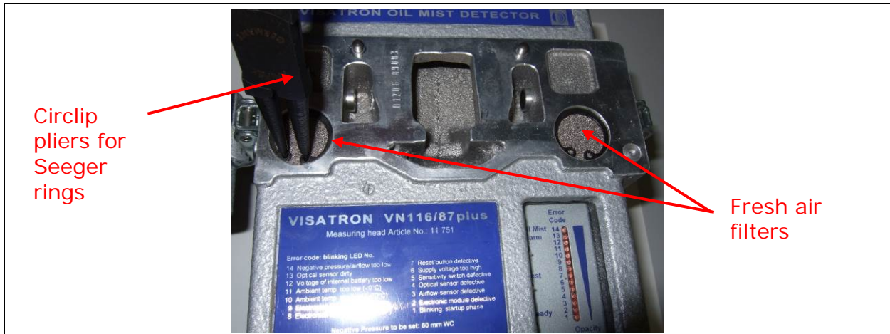
Figure 45: Exchange of the air filters
