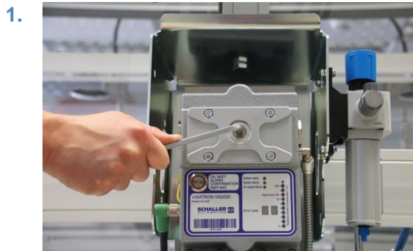
Figure 54: Inspection cover with screw plug
