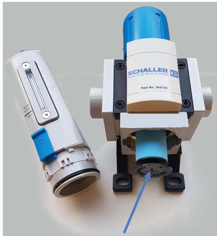
Figure 82: Filter control valve
