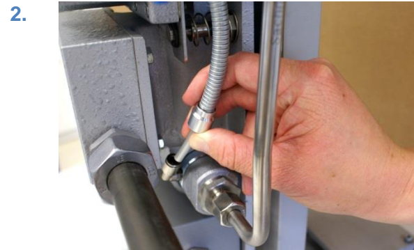
Figure 91: Detach the connecting hose from the venturi injector
