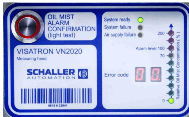
Figure 60: Measuring head display, in operating mode
