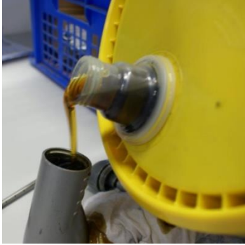
Figure 31: Fill lubrication oil into filling pump
