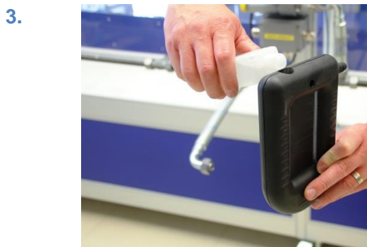
Figure 56: Fill U-tube manometer with water
