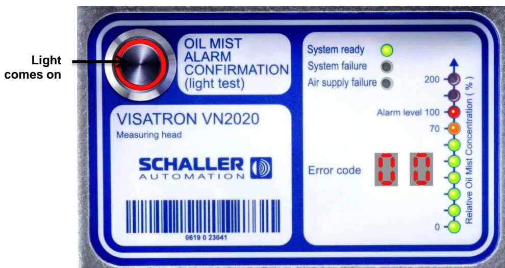
Figure 61: Display with detected oil mist
