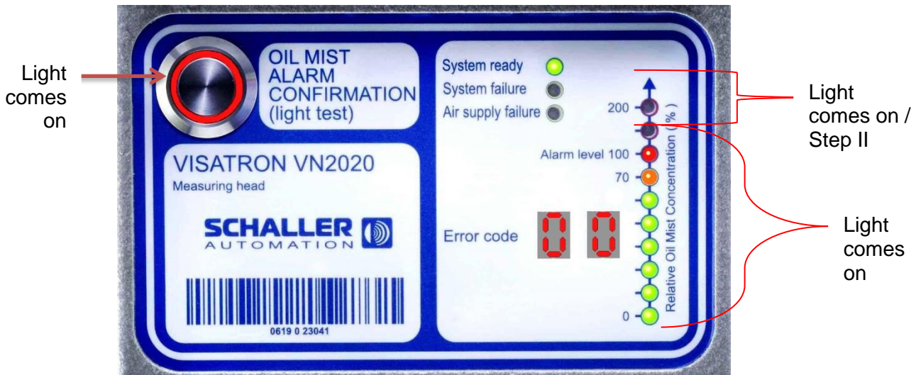
Figure 62: Example LED display with alarm
