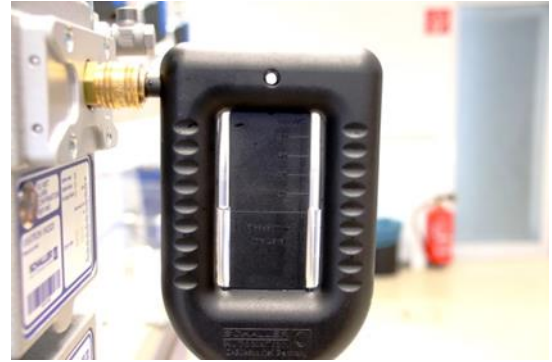
Figure 113: Setting the negative pressure at the measuring head
