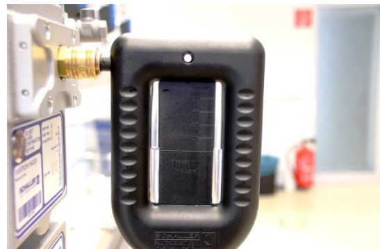
Figure 88: Check the negative pressure Check the negative pressure at the measuring head and readjust if necessary as per the steps in Section 7.10.1.
