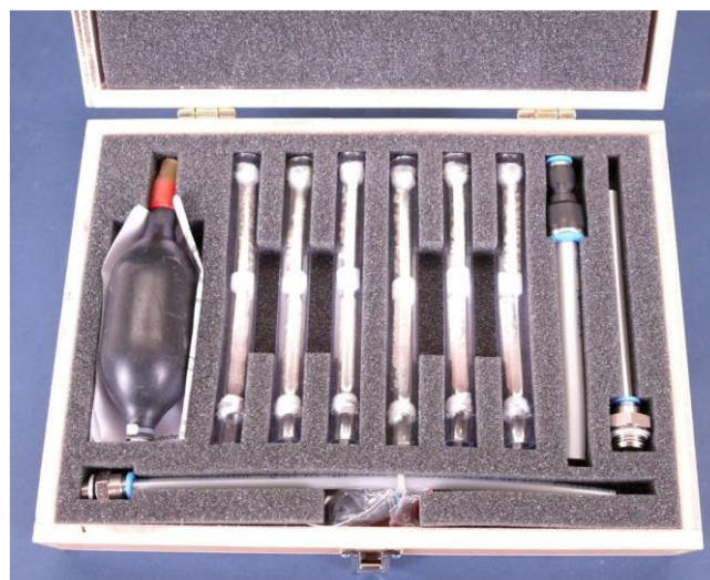
Figure 173: Smoke test box
