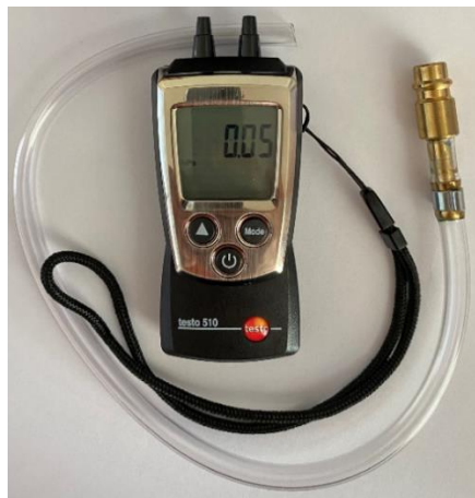
Figure 172: Differential pressure gauge
