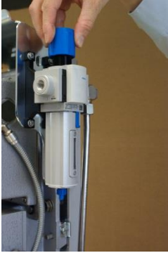
Figure 134: Release pressure in the filter control valve
