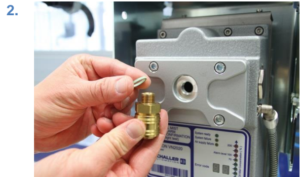
Figure 55: Inspection cover with quick-release coupling
