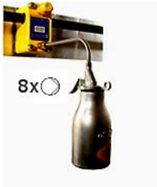
Figure 33: Pump lubrication oil
