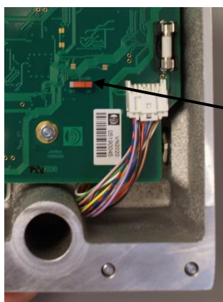
Figure 51: Switchable termination resistor
