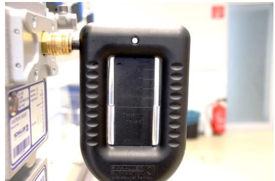
Figure 59: Negative pressure display on the U-tube manometer
