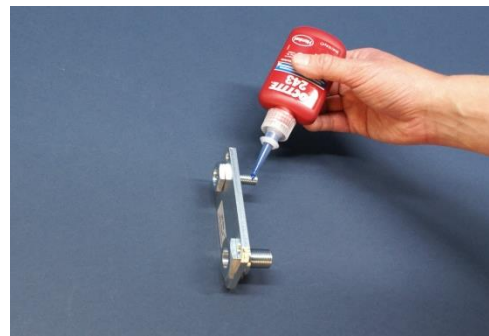
Figure 24: Screws with Loctite 243
