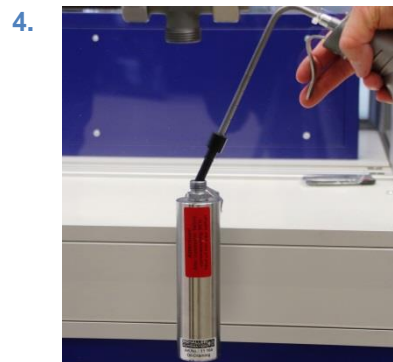
Figure 39: Filling the pipe siphon
