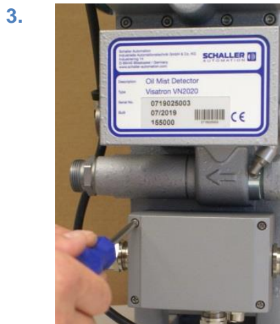
Figure 126: Remove the cover
