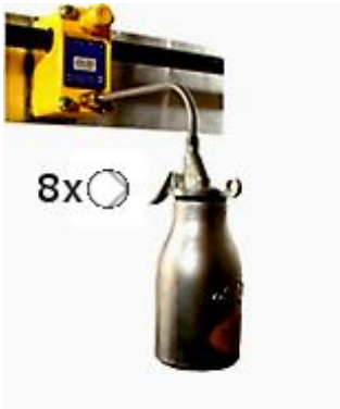
Figure 33: Pumping of lubrication oil
