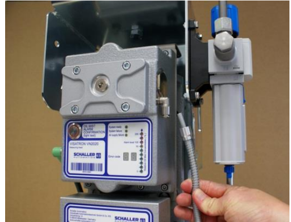
Figure 107: mounting of compressed air hose
