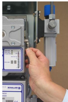
Figure 102: mounting of compressed air hose
