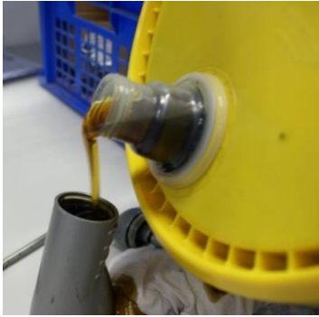
Figure 31: Filling of pump with lubrication oil
