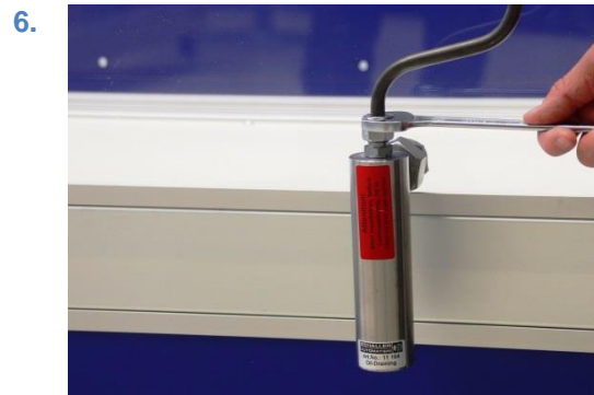
Figure 41: tightening of fitting
