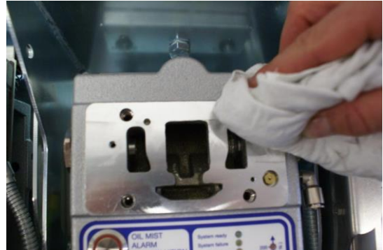
Figure 69: cleaning sealing surface
