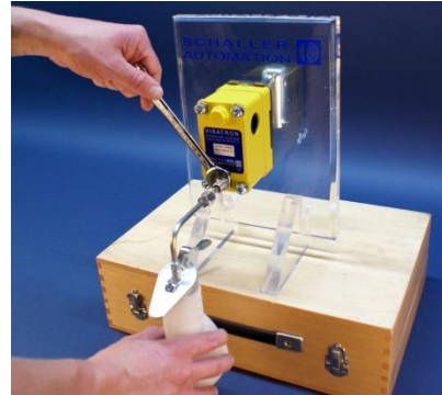
Figure 32: Installation of filling pump
