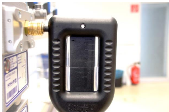
Figure 79: check negative pressure
