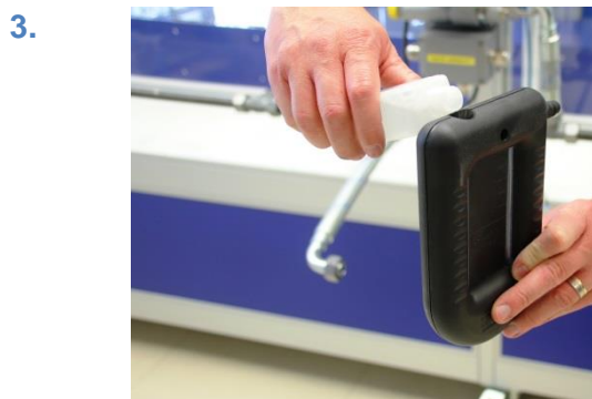
Figure 57: Fill U-tube manometer with water
