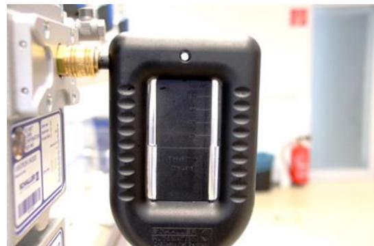
Figure 165: U-tube manometer on inspection cover
