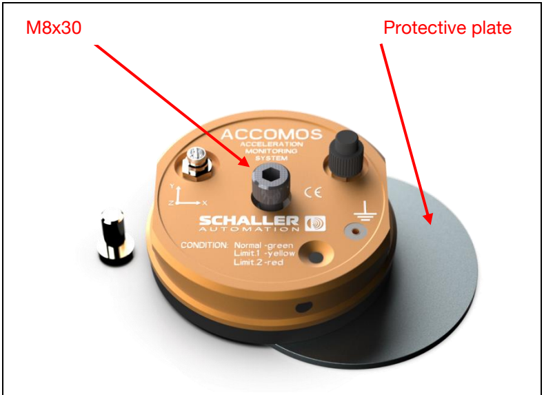
Illustration 2: Removing the protective plate with the M8x30 screw
