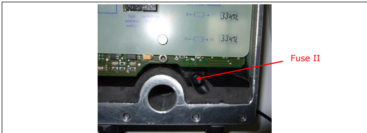
Figure 46 Fuse on the rear side of the measuring head
