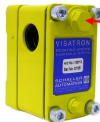
Figure 55: Test fog inlet on the siphon blocks
