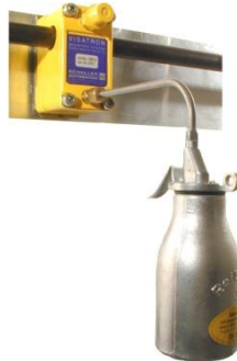
Figure 27: Filling pump inserted and fixed in the siphon block
