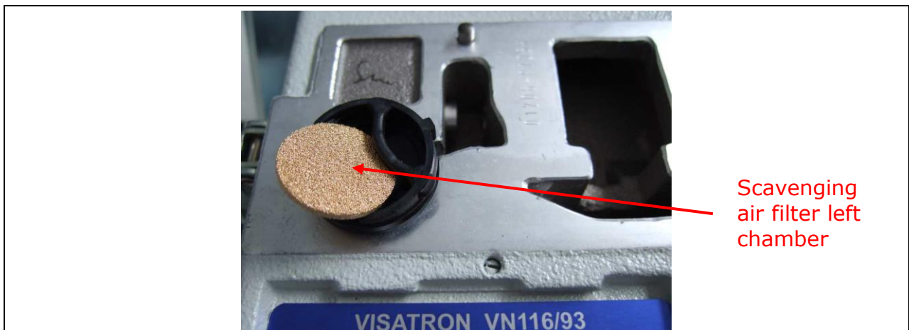
Figure 43: Exchange of the air filters
