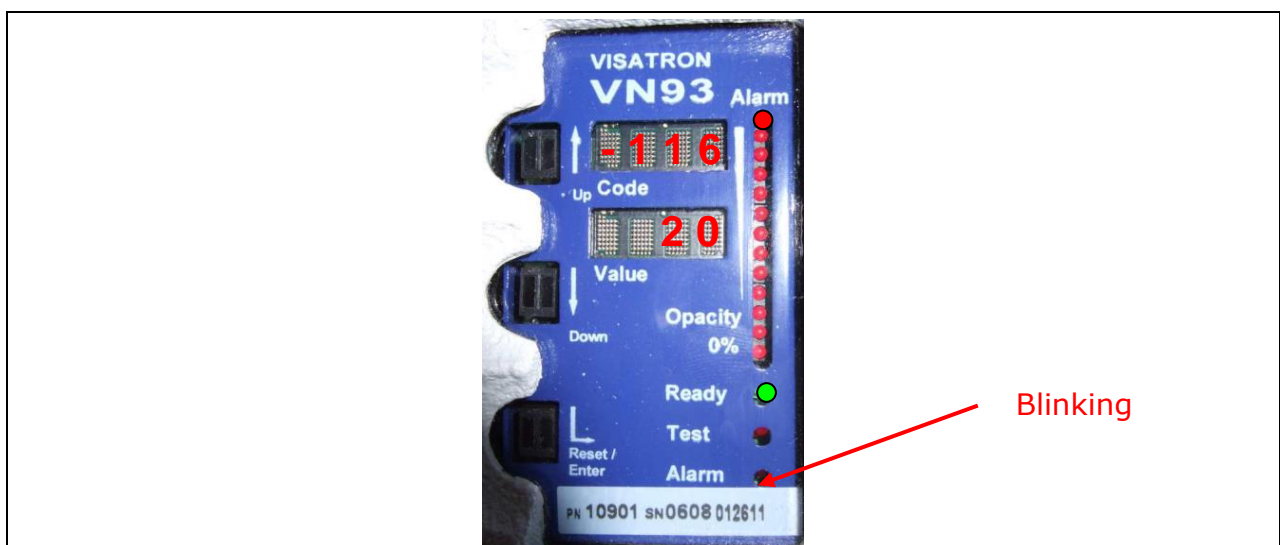
Figure 39: Example of an oil mist alarm state with 20% opacity
