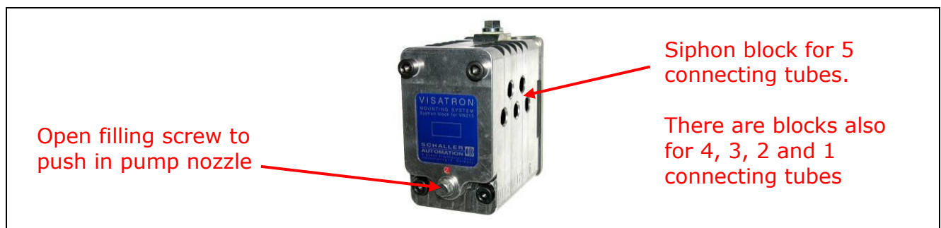
Figure 31: Siphon block VN280plus for 5 connecting tubes (5 holes on its side)
