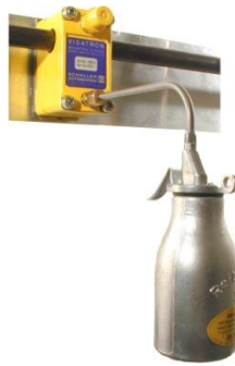
Figure 36: Filling pump inserted and fixed in the siphon block
