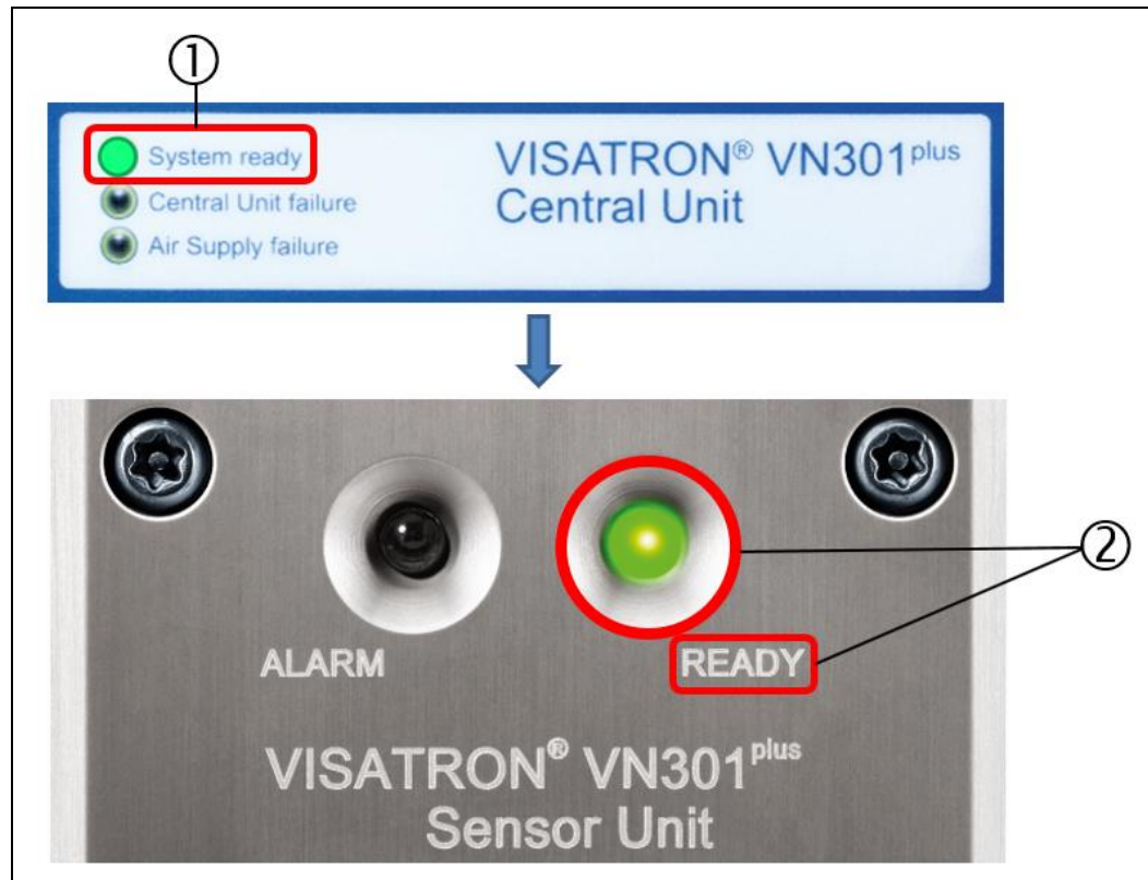
Fig.: 60 : System Ready on VN301 plus / VN301 plus Ex central unit and sensor unit
