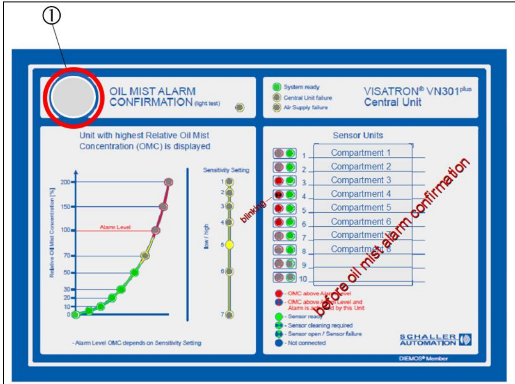
Fig.: 73 : VN301plus central unit: Confirm the oil mist alarm (only < 70% OMC)
