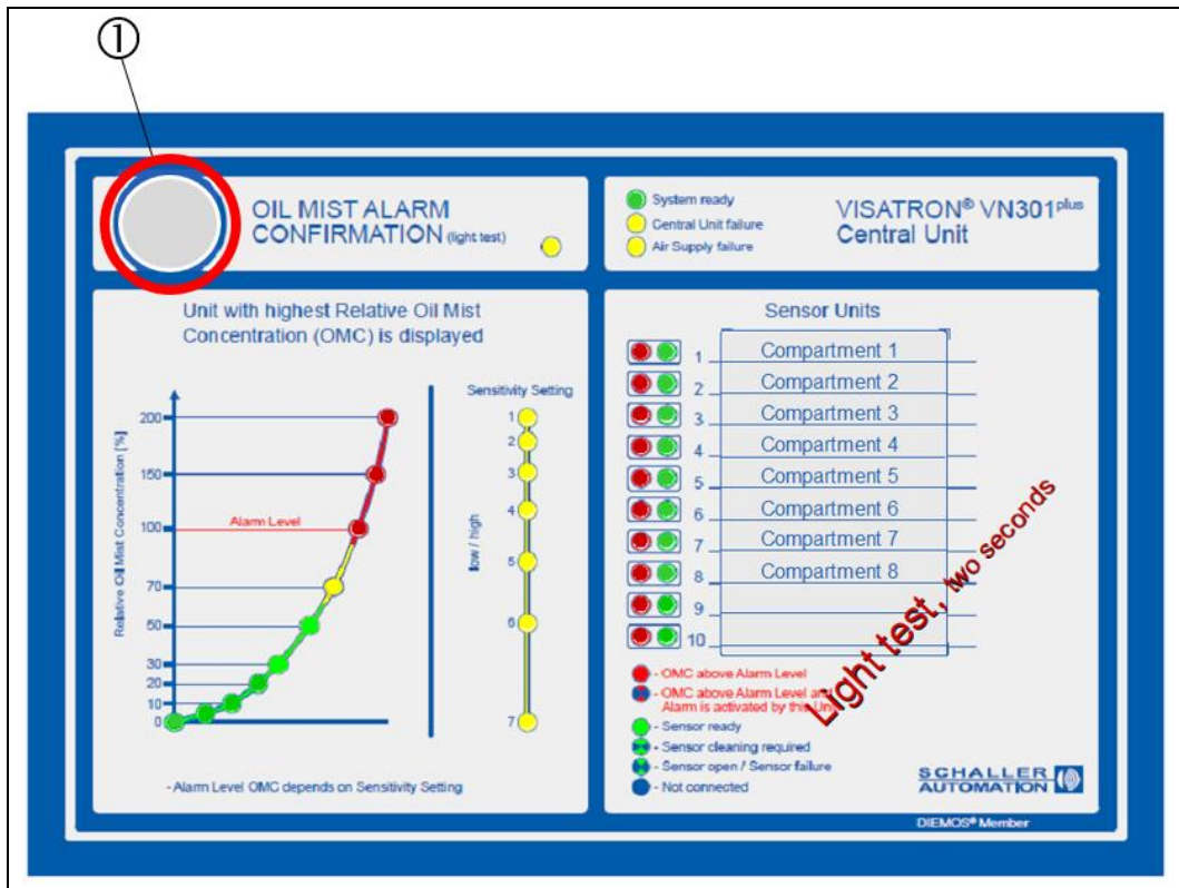
Fig.: 69 : VN301 plus central unit: LED check (light test)
