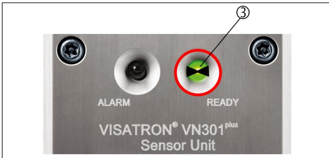
Fig.: 77 : “Sensor cleaning” status indicator on the VN301 plus / VN301 plus Ex sensor unit
