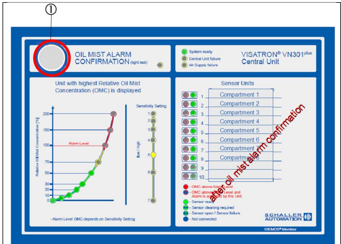
Fig.: 75 : VN301 plus central unit: Status display after confirming the oil mist alarm
