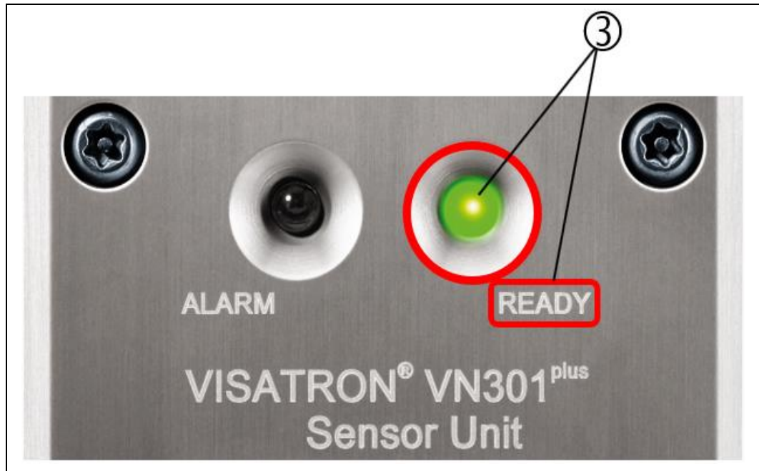
Fig.: 68 : "Sensor Ready" status indicator on the VN301 plus / VN301 plus Ex sensor unit
