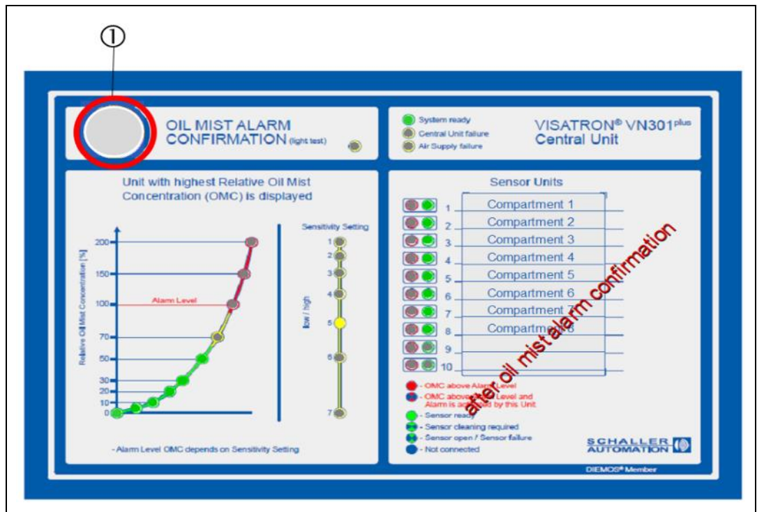
Fig.: 89 : VN301 plus central unit: Status indicator after confirming the oil mist alarm
