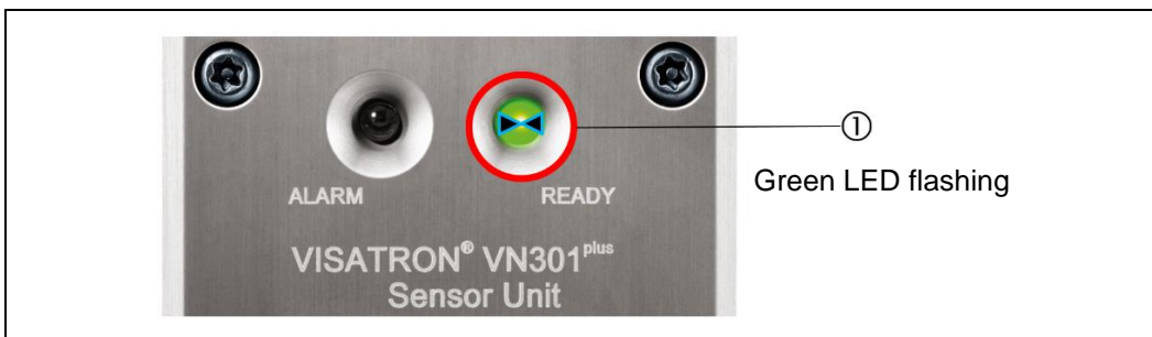
Fig.: 103 : VN301 plus / VN301 plus EX sensor unit: “Ready” status LED indicator
