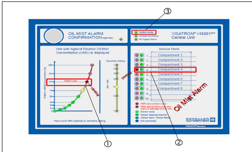
Fig.: 85 : VN301plus central unit: "Alarm" status indicator at 100% OMC (example 1)
