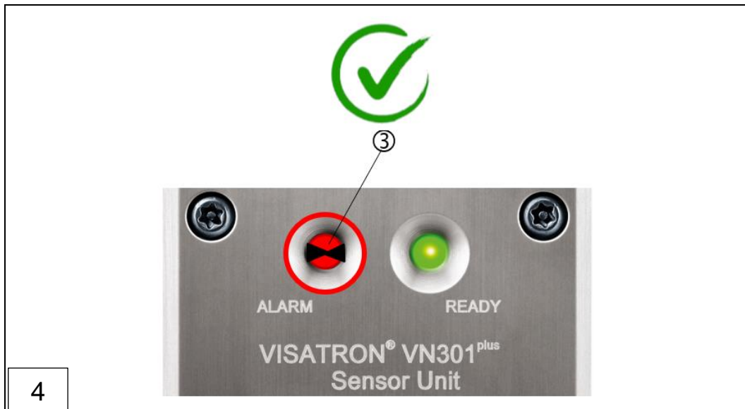
3: Red LED flashes when function test is successful
