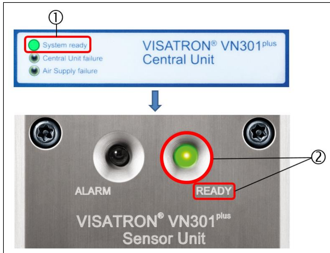
Fig.: 73 : System Ready on VN301 plus / VN301 plus EX central unit and sensor unit
